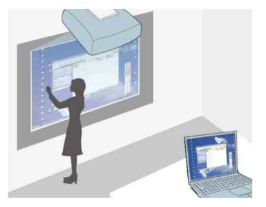
When the projector is connected to a computer with a USB cable, you can operate the computer from the projected screen using the interactive pens or your finger, just as you would with a mouse. You can navigate, select, and interact with your computer programs from the projected screen.
