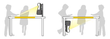
Make sure you select the correct **Projection** option in the projector's **Extended** menu according to the installation method being used.
