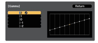
When you select a smaller value, you can reduce the overall brightness of the image to make the image sharper. When you select a larger value,
