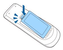
The Interactive pen uses one AA manganese battery, AA alkaline battery, or Eneloop (BK-3MCC) rechargeable battery. Replace the battery as soon as it runs out.
