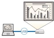
• Epson iProjection (Windows/Mac) to project up to four images at the same time by splitting the projected screen. You can project images from computers on the network, or from smartphones or tablet devices on which Epson iProjection is installed.
