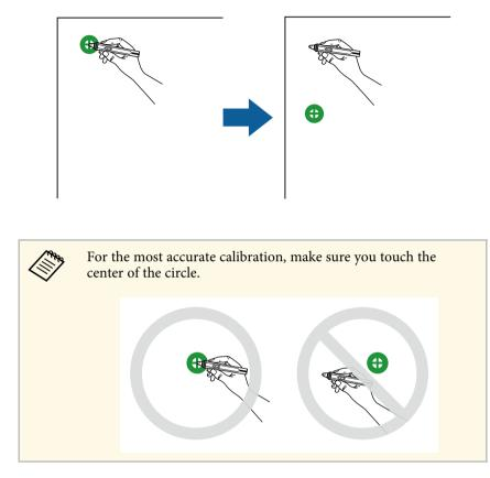
Touch the center of the next circle, then repeat. When you get to the bottom of the column, the next circle appears at the top of a new column.
