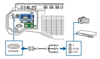
Tighten the screws on the VGA connector.
