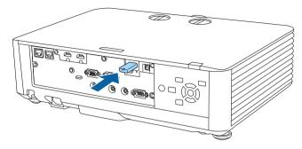
Attach the wireless LAN module cover, and secure it in place with the screw.
