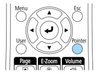
Use the arrow buttons to move the pointer on the screen. To move the pointer diagonally, press any pair of adjacent arrow buttons at the same time.
