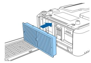
8 Close the air filter cover and tighten the screws.
