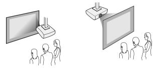
If you project from the ceiling or from the rear, select the correct **Projection** setting and, if necessary, turn on the **Inv Direction Button** setting and adjust the **OSD Rotation** setting.
