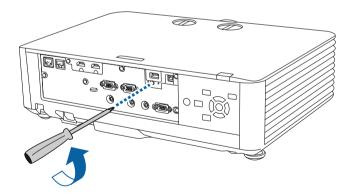
Connect the wireless LAN module to the USB-A port.
