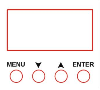
The MENU display will lock when NO buttons are pressed for 30 seconds. When the display locks, none of the control panel buttons will respond. To unlock the display, press and hold the MENU button 3 seconds to access the menu options once again.
