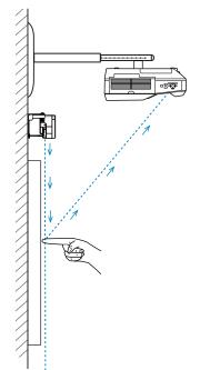
Adjust the angle of the laser light coming from the Touch Unit so that the projector can correctly detect the position of your finger.
