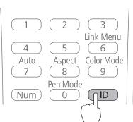
The ID set for the projector is displayed on the projected screen. The display turns off after approximately three seconds.
