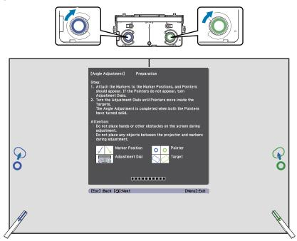
When you turn the adjustment dial counterclockwise, the pointer moves diagonally down away from the center of the projected image.
