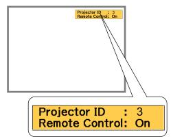
While holding down the [ID] button, press the button with the same number as the projector ID for the projector you want to operate
