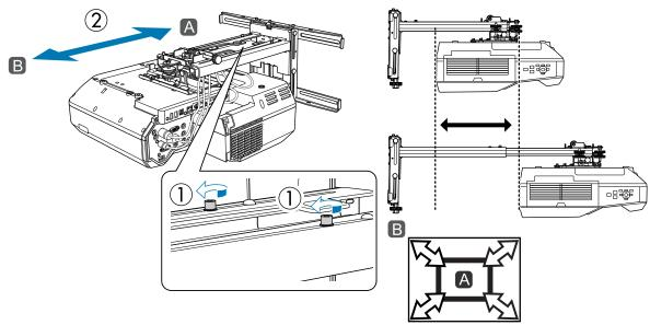
After you finish making adjustments, tighten the M4 bolts that you loosened.
