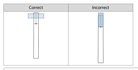
Do not place anything other than the markers near the projected image during angle adjustment. If other objects are on the projected image, angle adjustment may not be performed correctly.
