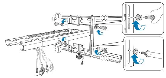
Adjust the vertical slide with the open-ended spanner, and align it with the standard position ( $\bigcirc$ )
