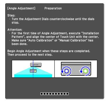
The next procedures are the same as for adjusting the angle (after step 11) when installing outside the whiteboard using the bracket.
