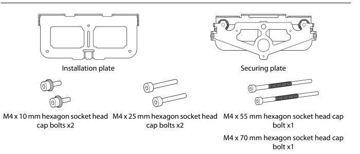
For the installation plate, you also need three commercially available 4 mm diameter wood screws, or three M4 anchor bolts.
