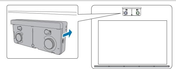
• Non-magnetic screens: Attach spacers and secure with M4 screws (x3).
