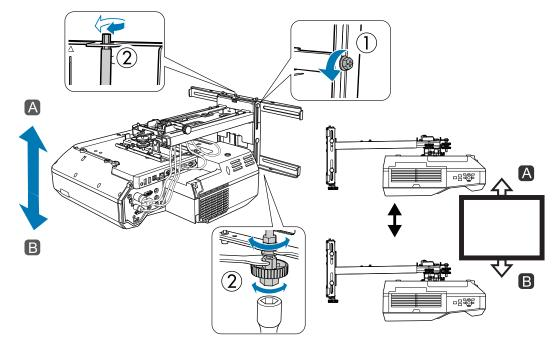
After you finish making adjustments, tighten the M6 bolt that you loosened.
