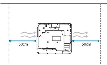
• When installing two or more projectors in parallel, make sure the temperature of the surrounding environment is less than 35°C.
