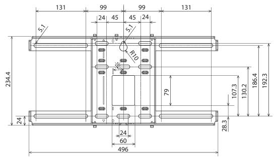
\* The offset value for the position of the center of the projected image and the center of the wall plate is 27 mm.
