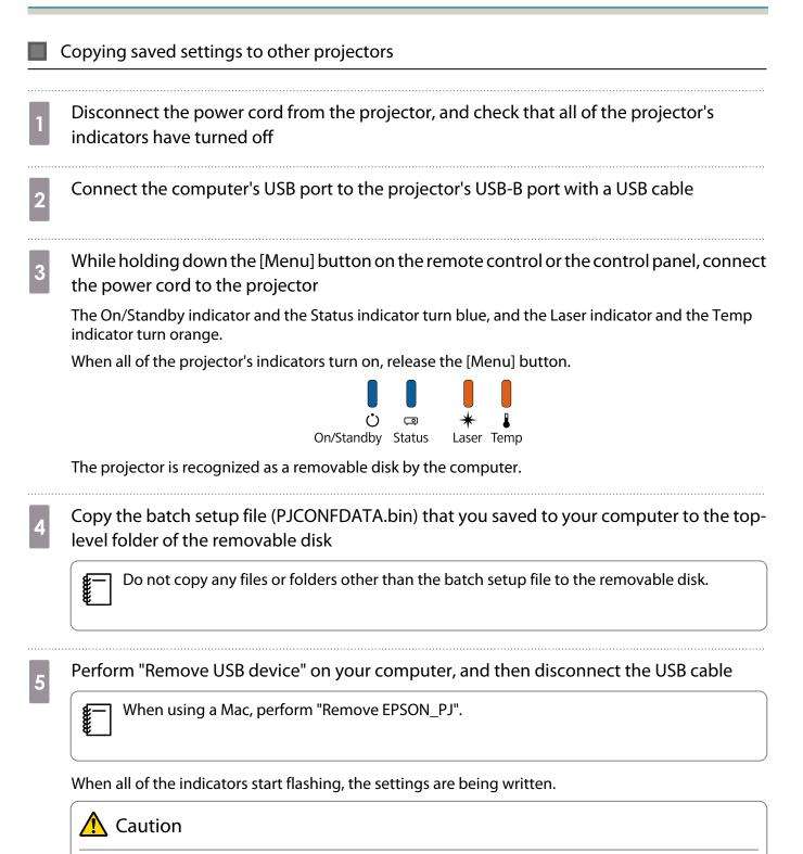
Do not disconnect the power cord from the projector while the settings are being written. If the power cord is disconnected, the projector may not start correctly.
