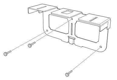
Attach the securing plate to the rear of the Touch Unit with the two M4 x 25 mm bolts supplied
