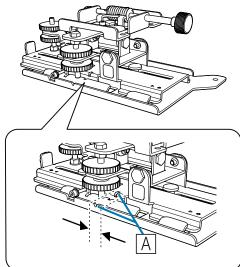
If the standard position ( $\boxed{A}$ ) is not correct, loosen the M4 bolt and adjust the position of the slide plate. When you have finished making adjustments, tighten the bolt.
