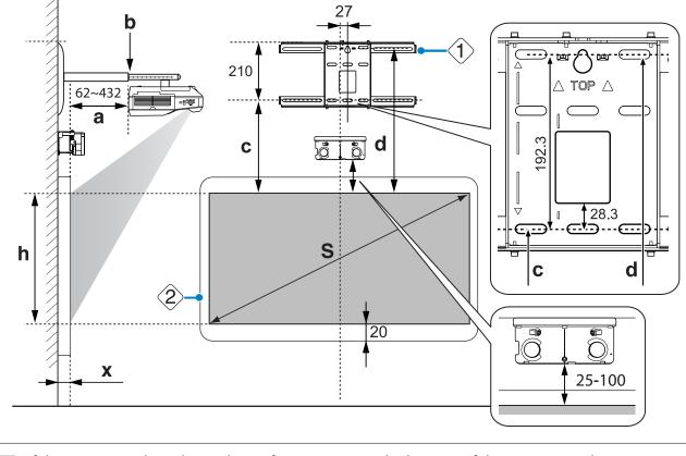
When the Touch Unit is installed outside the whiteboard (using the Touch Unit Bracket)
