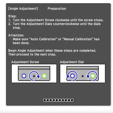
Turn the adjustment screw for the Touch Unit fully clockwise using the hexagon wrench supplied with the setting plate
