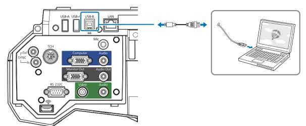
Necessary cables when installing two projectors in parallel and using the Easy Interactive Function (EB-710Ui only)
