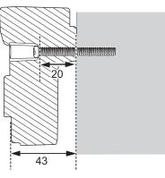
Screw hole cross-section
