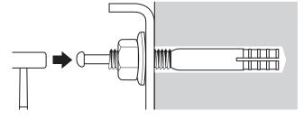
Tighten the nut with a commercially available spanner to secure the wall plate to the wall
