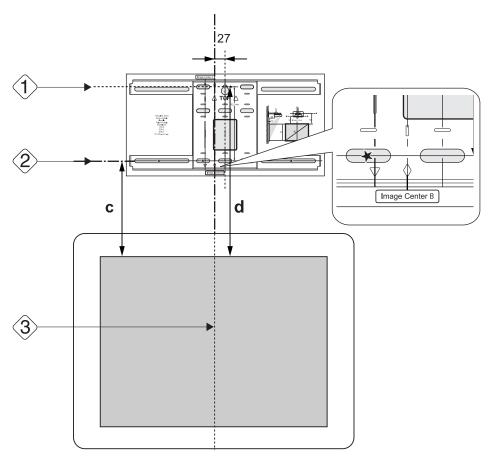
3 Drive a commercially available M10 screw into the position of the temporary screw hole for the wall plate
