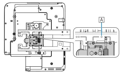
The distance from the top of the projected image to the bottom wall plate installation screw hole (c) is the number given when the vertical slide is set to the standard position (B).
