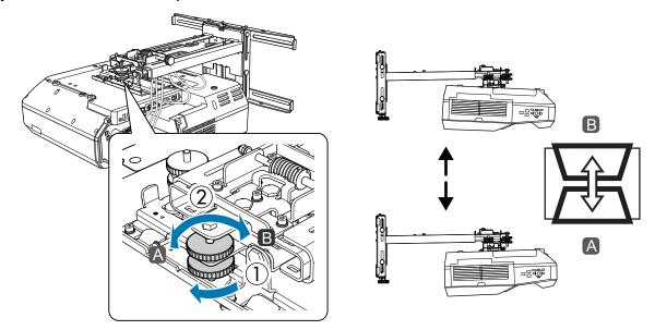
After you finish making adjustments, tighten the adjustment dial at the bottom.
