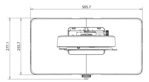
When installing the wall plate cover, you need a space of approximately 263 mm from the center of the wall plate to the left side, and approximately 253 mm to the right side.
