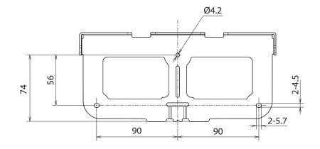
When the Touch Unit is installed (side)
