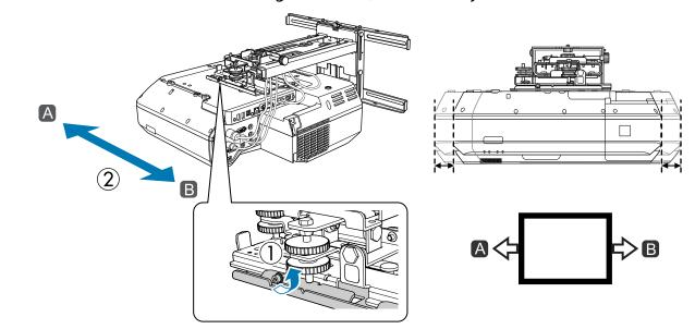
After you finish making adjustments, tighten the M4 bolt that you loosened.
