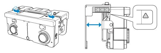
Secure the Touch Unit and the installation plate with the hexagon socket head cap bolt
