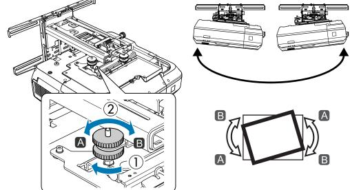
After you finish making adjustments, tighten the adjustment dial at the bottom.
