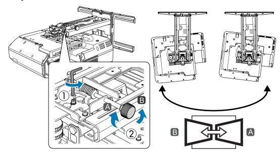
After you finish making adjustments, tighten the M4 screws that you loosened.
