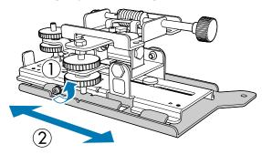
Secure the 3-axis adjustment unit and the slide plate to the base of the projector with the M4 x 12 mm bolts (x4) supplied
