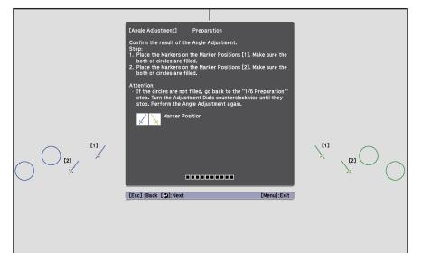
Place the markers at the top marker positions [1] ( $\checkmark$ ) ( $\checkmark$ )
