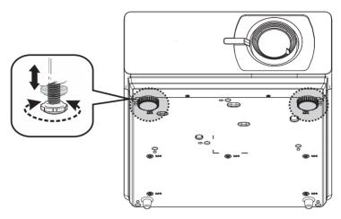
The projector is equipped with two adjuster foot. It changes the image height and vertical projection angle. Screw the adjuster foot to fine tune the angle until the image is positioned where you want it.
