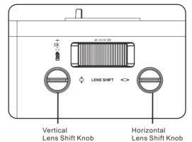
The Lens Shift feature provides a lens shift function that can be used to adjust the position of the projected image either horizontally or vertically within the range detailed below.
